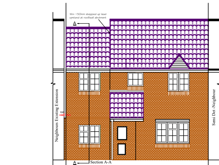
Proposed - West Facing Front Elevation Section A-A - NTS
